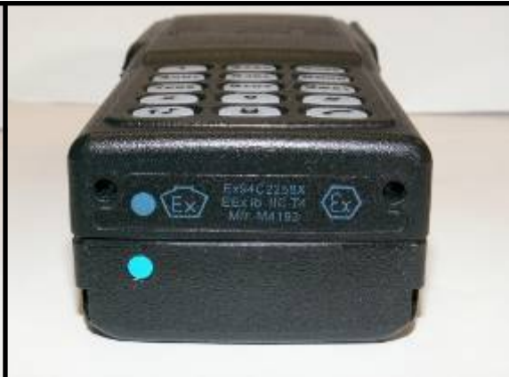
Fig 4. Cenelec Radio & Battery correctly installed
