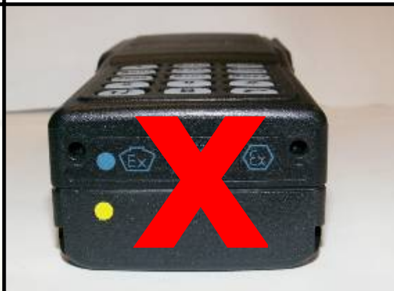
Fig 6. Cenelec Radio with incorrect ATEX Battery
