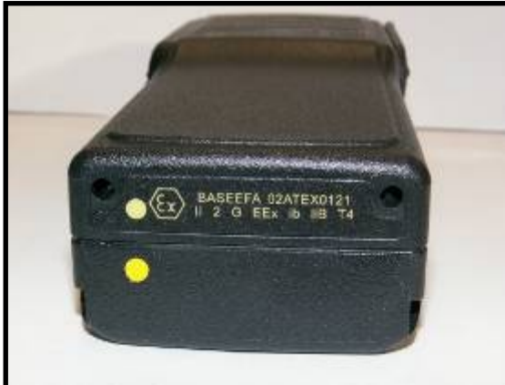
Fig 3. ATEX Radio & Battery Correctly Installed
